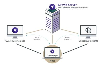
The signaling process, as per the WebRTC terminology, refers to the exchange of streaming media (audio/video codecs) and network capabilities between endpoints (the clients). This operates over WebSocket on Drovio.
