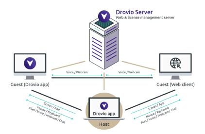
P2P connections then operate between clients. A live video stream of the host screen or app is sent to the guests, along with any audio stream (microphone or system audio). Guests may share their microphones too and send mouse/keyboard inputs. Drovio Server is not involved during the screen sharing session, except to collect various statistics to improve user experience as described below.
