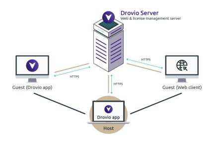
Authentication on Drovio operates over HTTPS (TLS v1.2). WebSocket connections are initiated between Drovio Server and the clients to handle the overall signaling process.
